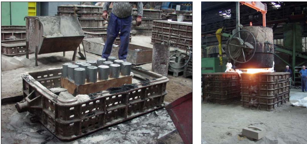
Fig. 2-3 The moulding of the block with chills on one side and its pouring
