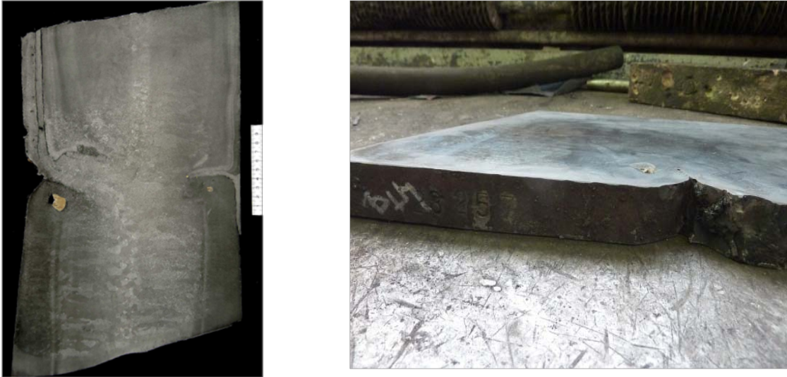
Fig. 8-1a A plate taken from the breakout area
