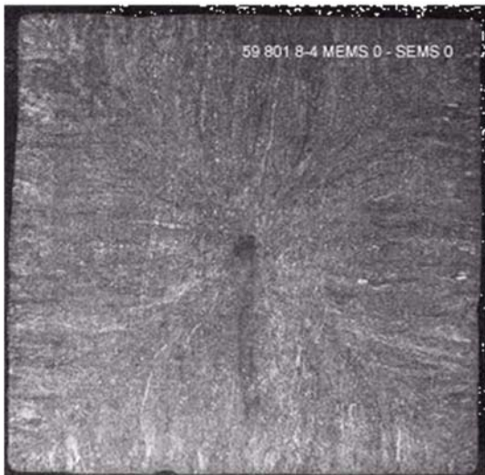
Fig. 9-2 The growth of dendrites without EMS – mode 2A (up) and mode 2B ( Tab. 9-2 )
