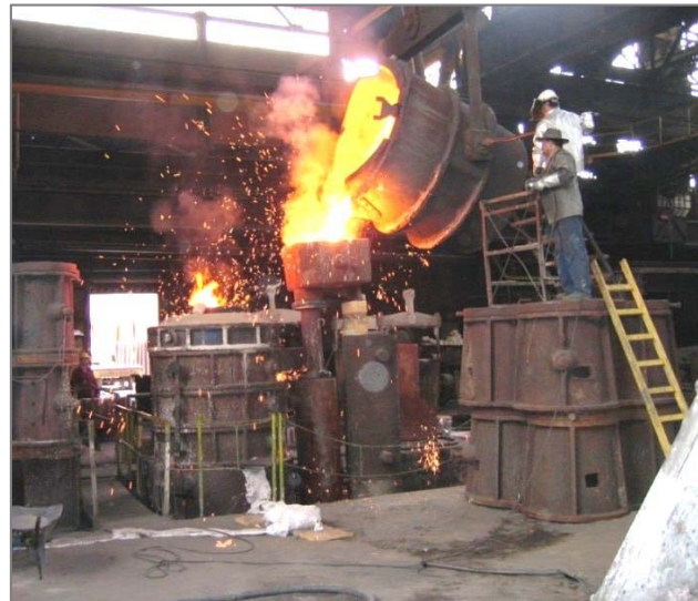
Fig. 3-3 The pouring of the roller
