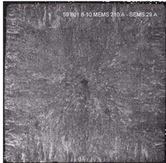
Fig. 9-3 The growth of dendrites using MEMS and FEMS-mode 4A (up) and mode 5B ( Tab. 9-2 )
