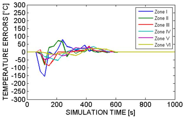
Figure 14: Surface temperature errors: case with control by means of PID regulator
