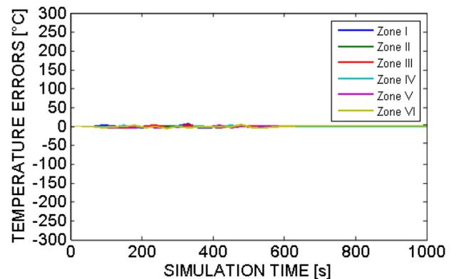
Figure 18: Surface temperature errors: case with control by means of model predictive control system
