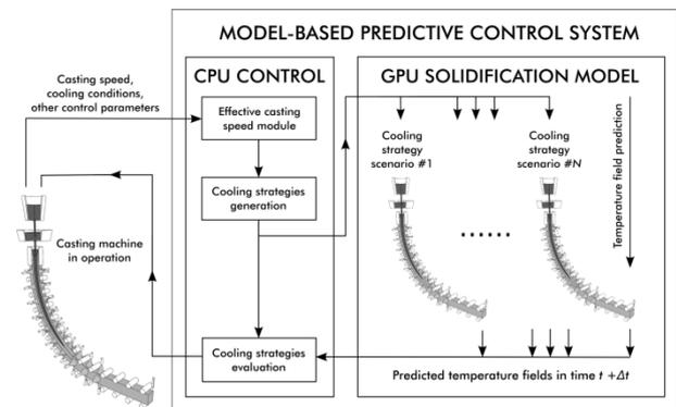
Figure 5: Scheme of parallel model predictive system
