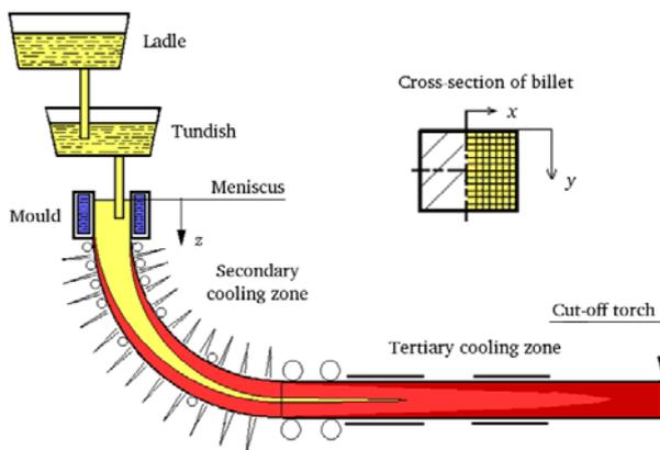
Figure 1: Scheme of the billet casting machine
