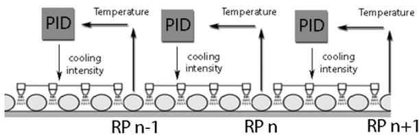
Figure 3: PID regulation of secondary cooling
