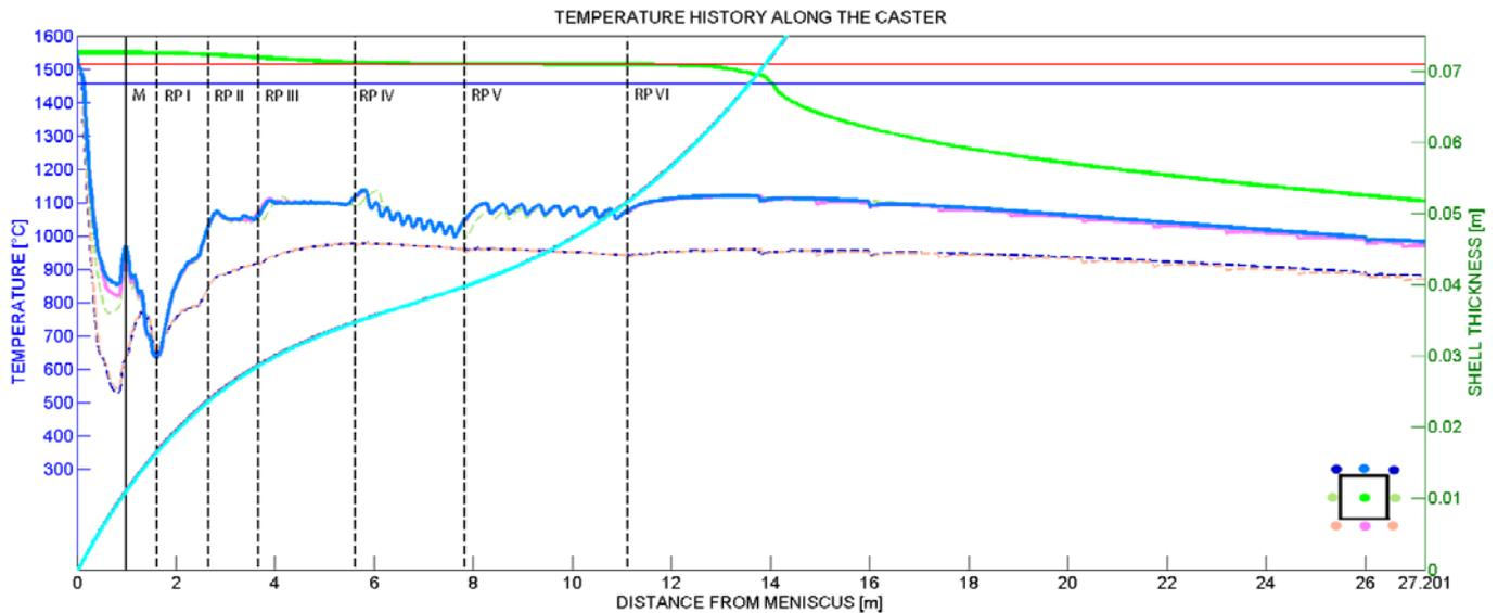
Figure 6: Steady state temperature field, which was considered as optimal solution for regulation
