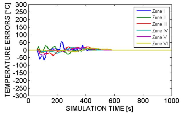
Figure 16: Surface temperature errors: case with control by means of fuzzy regulator
