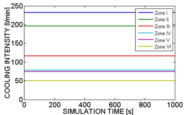
Figure 9: Water flow volumes: case with no regulation of secondary cooling
