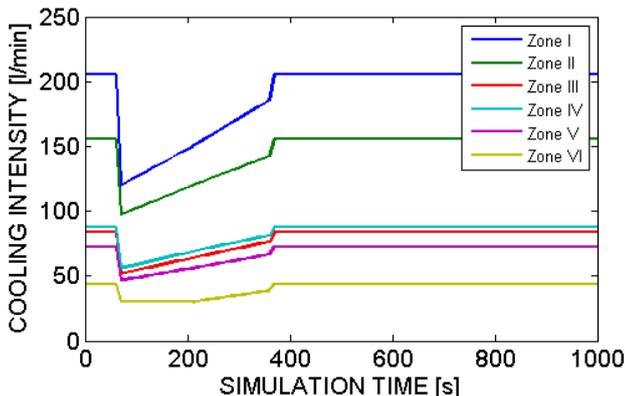
Figure 11: Water flow volumes: case with control by means of cooling curves
