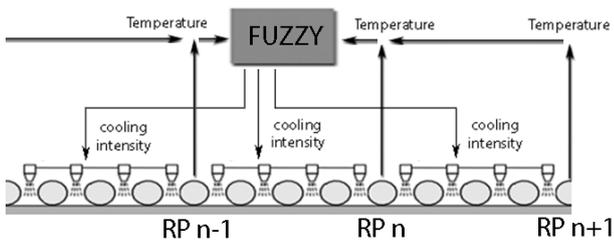
Figure 4: Fuzzy control system in secondary cooling
