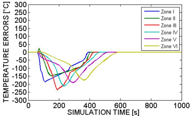
Figure 10: Surface temperature errors: case with no regulation of secondary cooling
