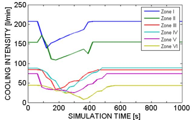
Figure 17: Water flow volumes: case with control by means of model predictive control system
