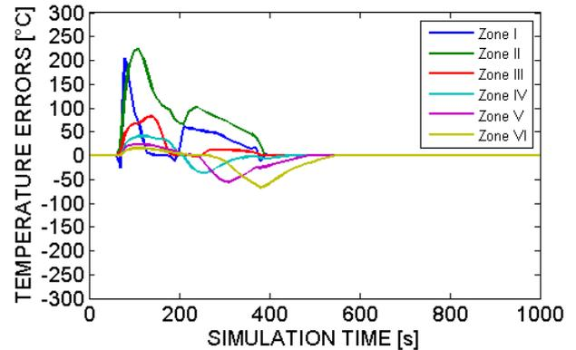
Figure 12: Surface temperature errors: case with control by means of cooling curve
