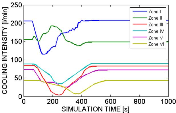
Figure 15: Water flow volumes: case with control by means of fuzzy regulator
